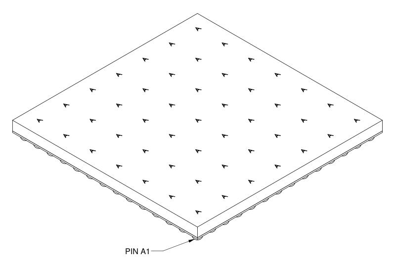
WLP IS LASER MARKED WITH A SINGLE LETTER REPEATED ACROSS THE TOP SURFACE.
