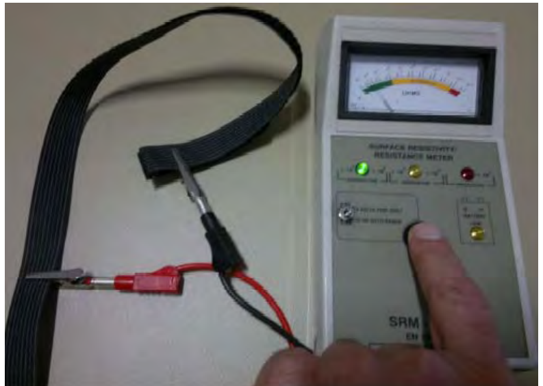
VGRIP tray strap under test using a Conductivity meter. The green reading on meter is > 10^3 Conductive < 10^6 Ohms
