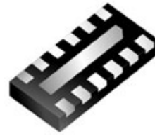
QFN Rectangle Quad Flat No Lead Page 7
