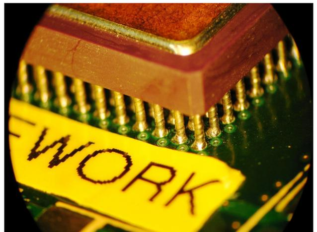
**Figure 19 - Close up view of Solder joint generated by rework process**
