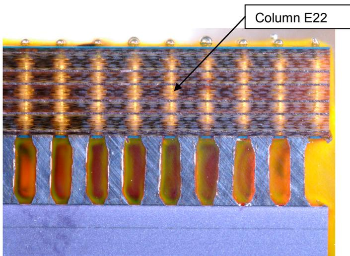
**Figure 25 - Suspected Via**
