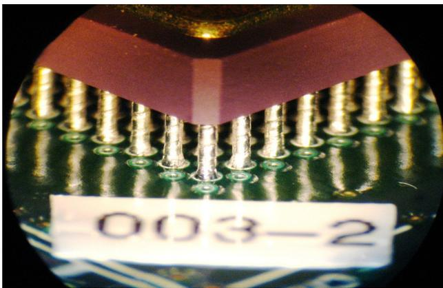
**Figure 13 - Close up view of CGA Columns Soldered to PWB**
