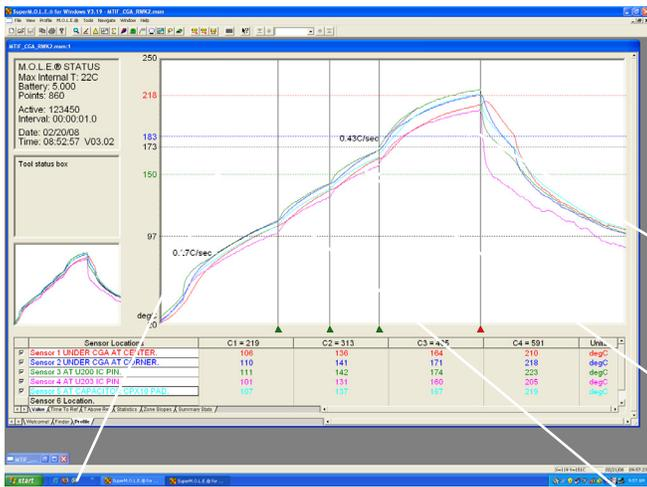
**Figure 7 - Graphical representation of thermal profile**
