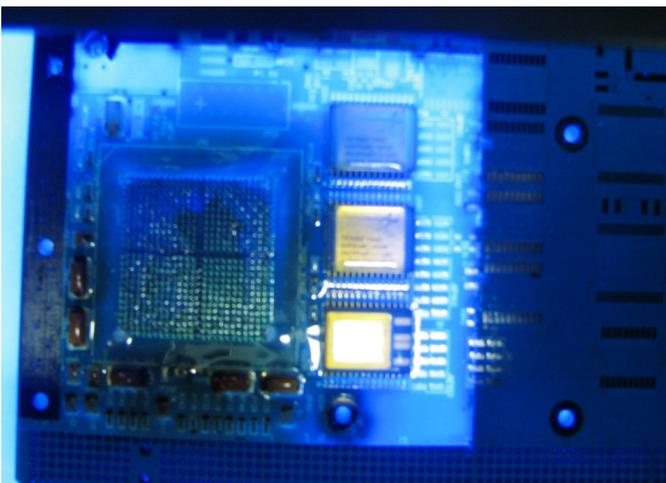
**Figure 16- Conformal Coated Board as viewed under UV light**
