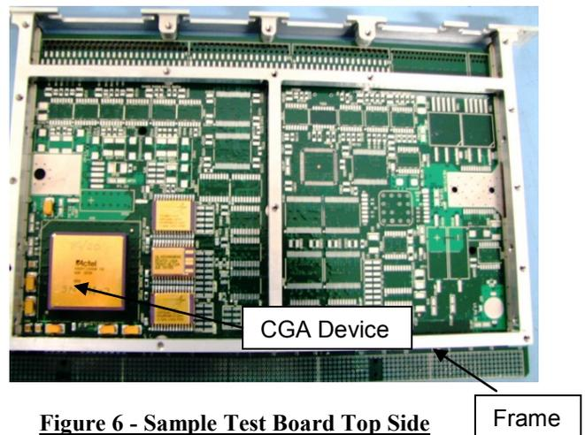
**Figure 6 - Sample Test Board Top Side**
