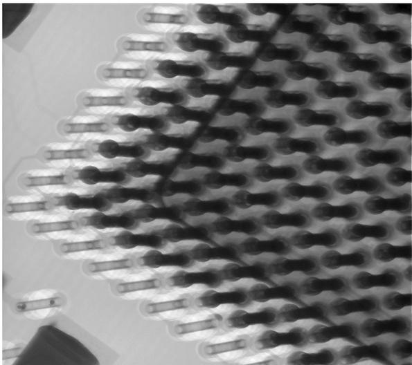
**Figure 21 - Tilted X-Ray view of solder joints after rework**
