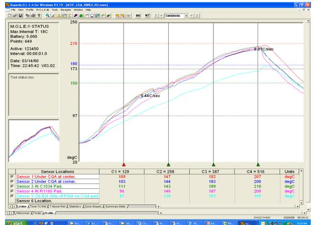
**Figure 8 Graphical representation of thermal profile for Second Series of Temperature Tests**
