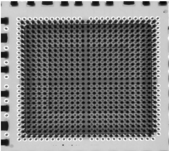
**Figure 20 - X-Ray view of solder joints after rework**
