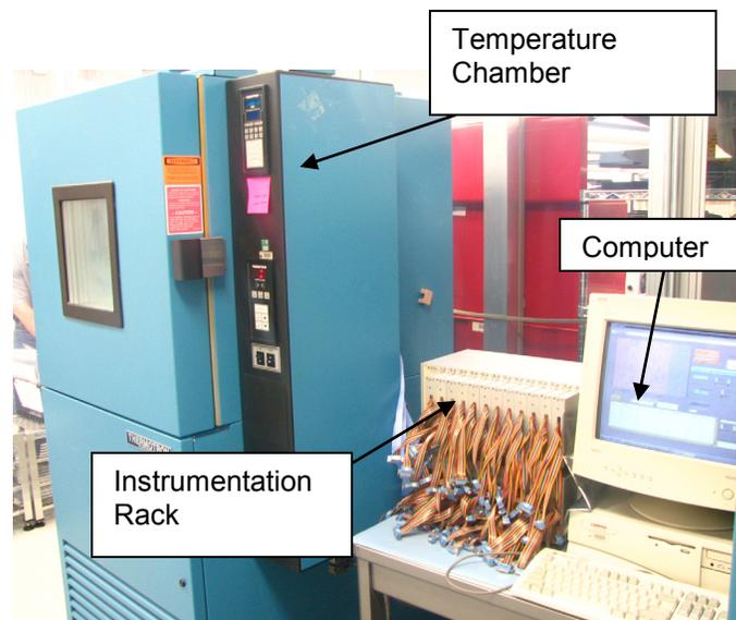
**Figure 26 - Thermal Cycling Test Setup**
