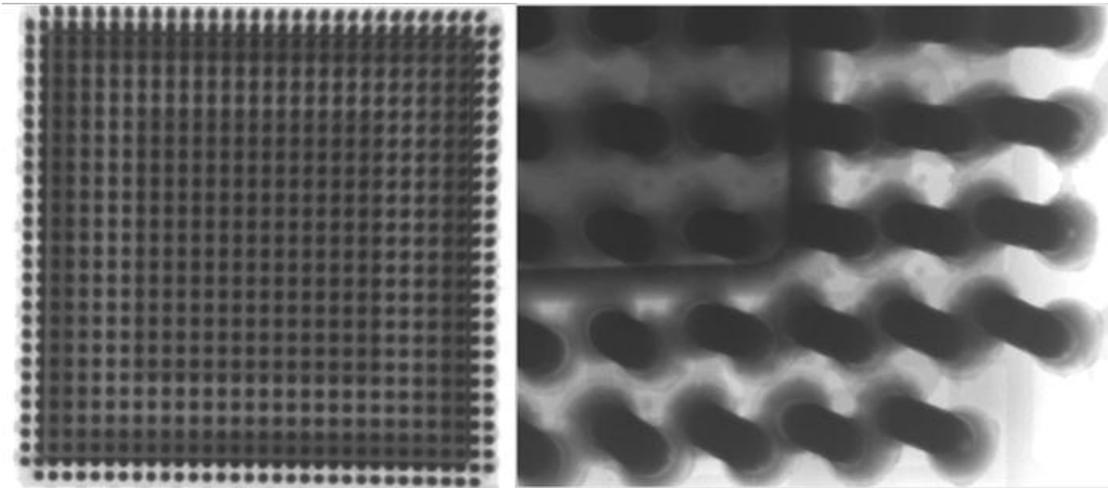
**Figure 6:** X-ray imaging of the CCGA 1152 assembled board prior to thermal cycling
