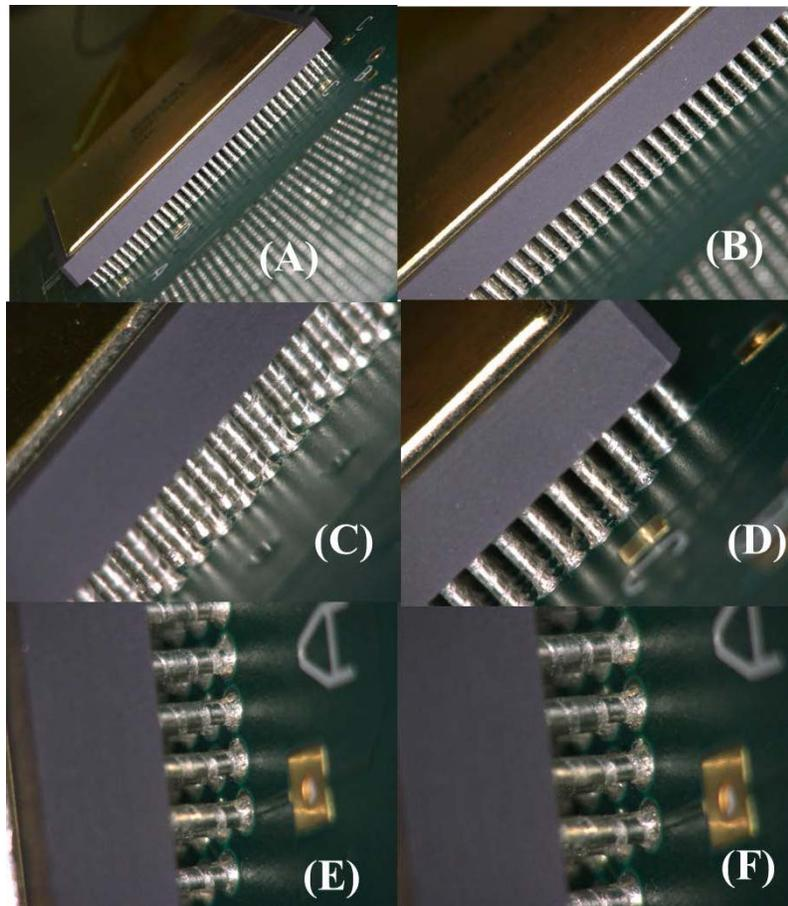
**Figure 14:** Microscopic images of the Actel CCGA 1272 package after 258 thermal cycles from -185°C to 125°C
