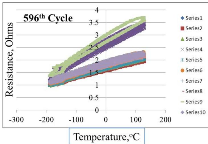
Figure 12: Resistance of all daisy chains during the 596<sup>th</sup> cycle.
