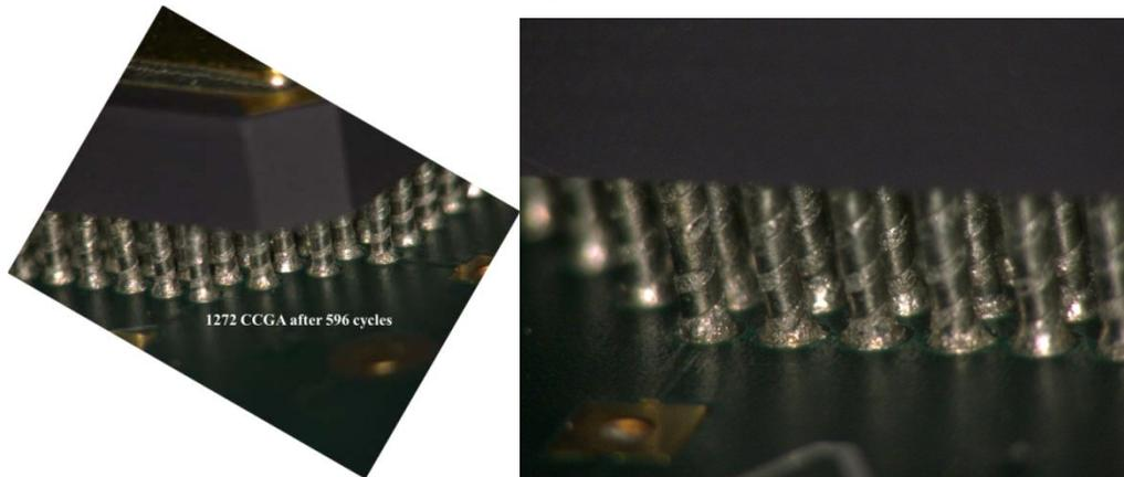
**Figure 17:** Microscopic images of the column which have not been bent due to thermal cycling (CCGA 1272) for 596 cycles
