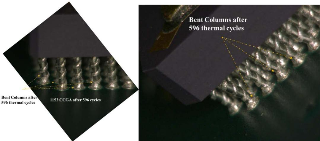
**Figure 16:** Microscopic image of the column which have been significantly bent due to thermal cycling. (CCGA1152) for 596 cycles
