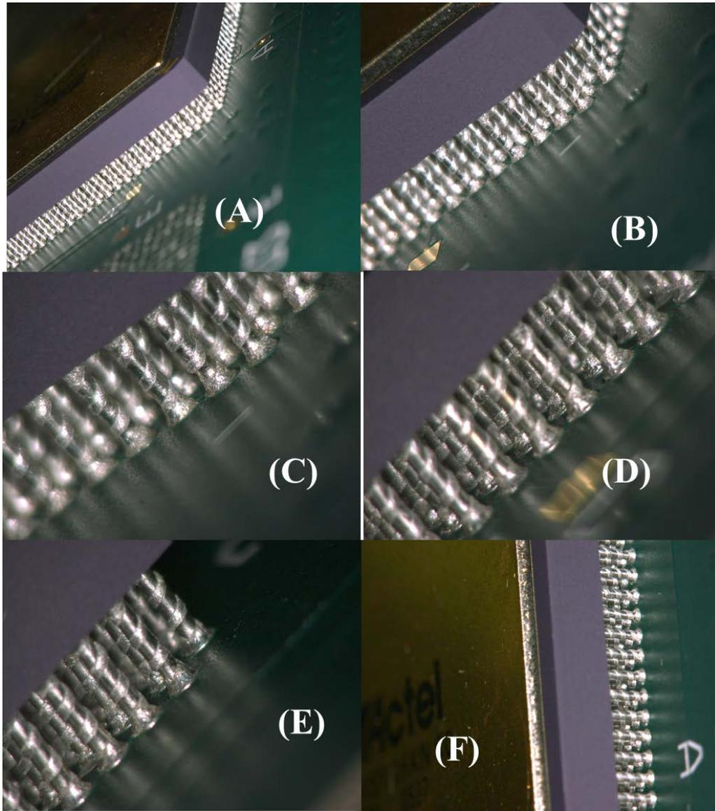
**Figure 13:** Microscopic images of the Actel CCGA 1152 package after 258 thermal cycles from -185°C to 125°C
