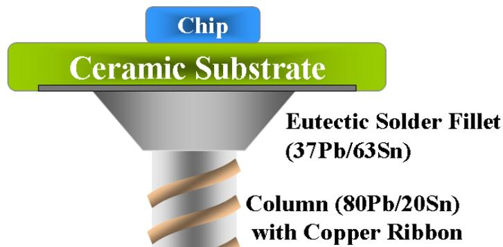
**Figure 1:** Schematic of a Column in a CCGA Package
