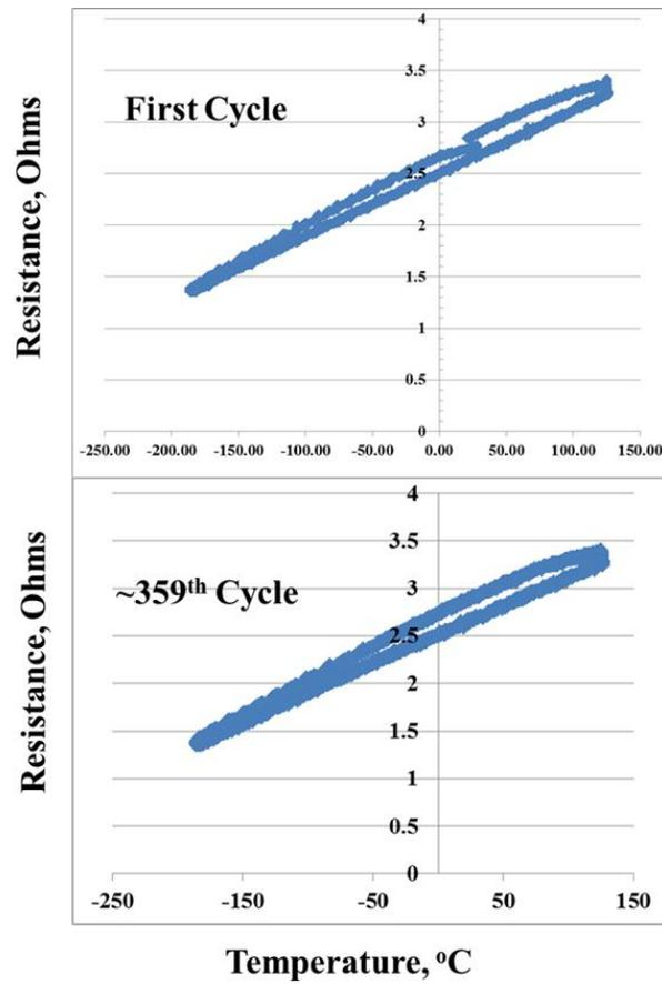
**Figure 9:** Resistance of one daisy chain during the first cycle and also during the 359<sup>th</sup> cycle.
