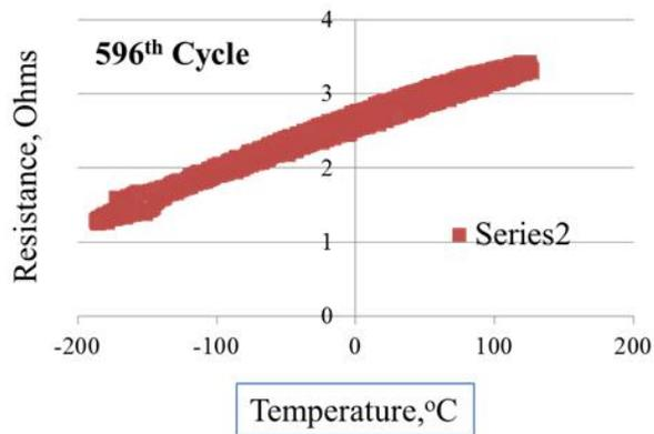
**Figure 10:** Resistance of one daisy chain during the 596<sup>th</sup> cycle.
