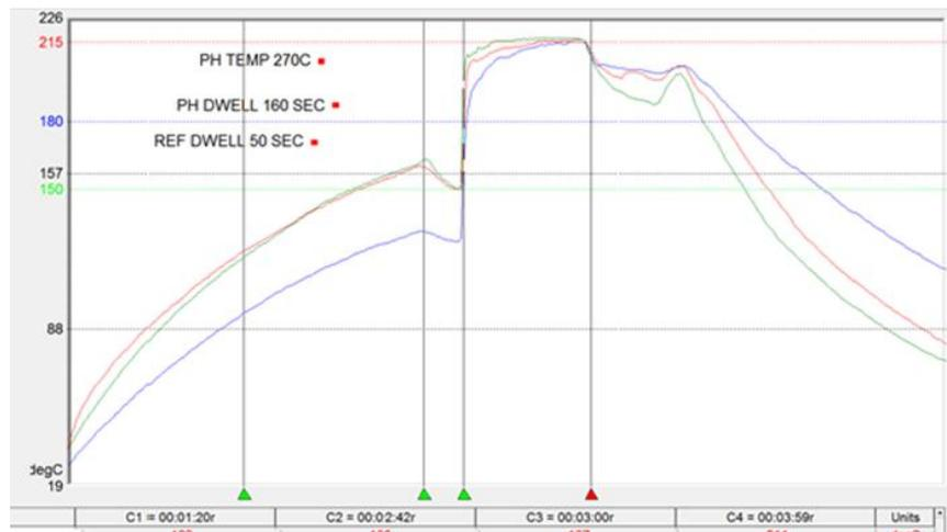
**Figure 4:** Reflow profile that was used to reflow CCGA1152 and CCGA1272 packages.
