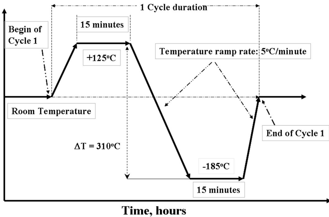
Figure 8: Extreme Temperature Thermal Cycling Profile used in this study
