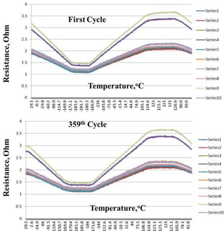
Figure 11: Resistance of ten daisy chains collected during the first cycle and also during the 359<sup>th</sup> cycle.
