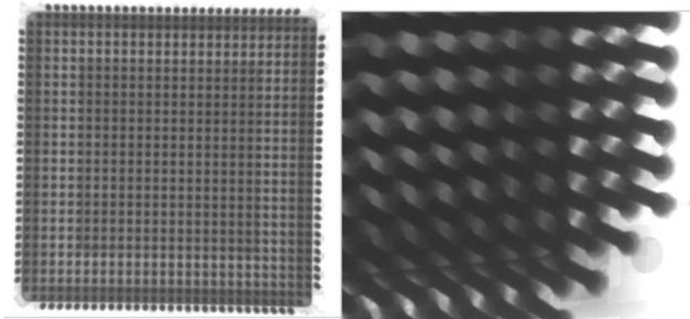
Figure 7: X-ray imaging of the CCGA 1272 assembled board prior to thermal cycling
