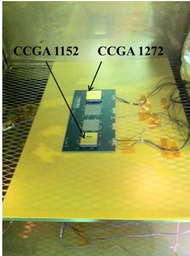
**Figure 5:** Optical photograph of the test board assembled with CCGA1152 and CCGA1272 packages
