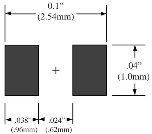
Tolerance  $\pm .004''$  ( $\pm .1\text{mm}$ )
