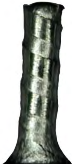
Free end Solder Bump Before Planarizing
