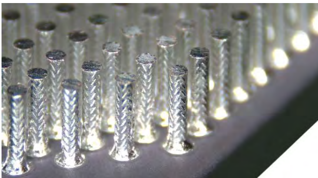
Fig. 3: Copper Braided Solder Columns attached to daisy chain test vehicle ceramic package.
