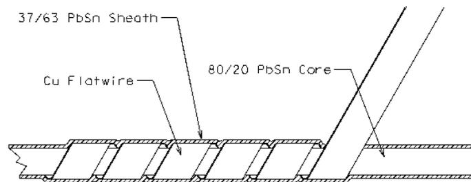
**Figure 2. Six Sigma Services solder column construction.**
