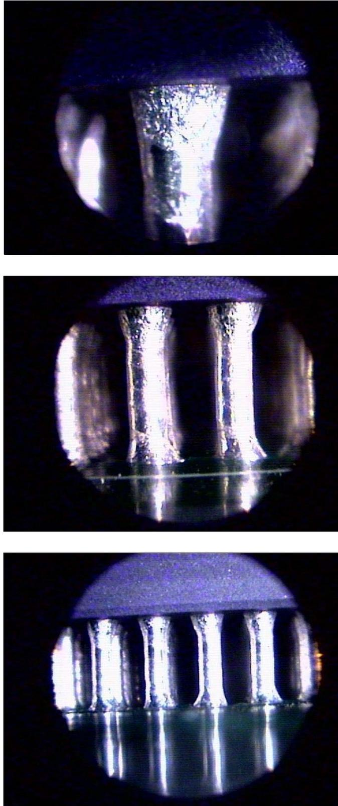
**Figure 5. Post-HASS solder column images.**
