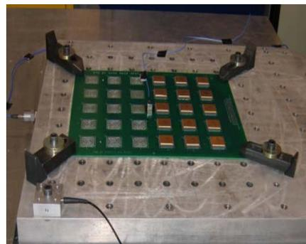
**Figure 1. Board level test setup.**
