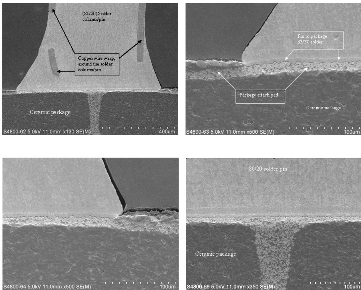
**Figure 7. Cross section SEM images of unstressed package.**
