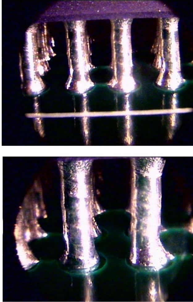
**Figure 4. Zero stress solder column images.**
