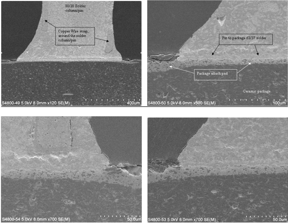
**Figures 8. Cross section SEM images of stressed package.**
