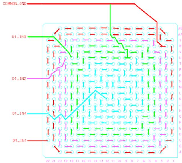
**Figure 3. 472 pin CCGA daisy chain structure.**
