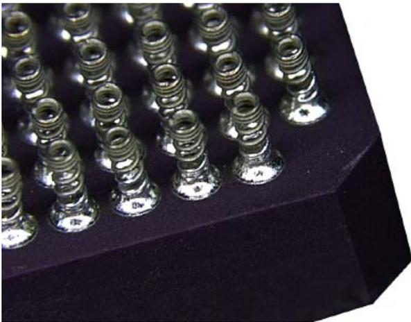
**Figure 6.** Micro-Coil Springs attached to CCGA.
