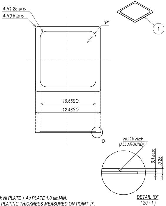
**NOTES** 1. FINISH: Ni PLATE + Au PLATE 1.0 μmMIN. PLATING THICKNESS MEASURED ON POINT 'P'.
